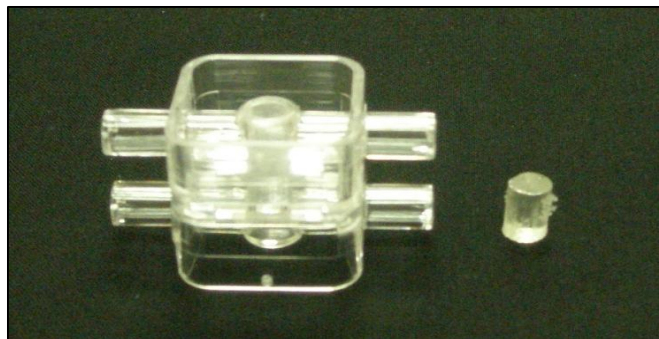
Histology sample in polymerized glycol methacrylate (shown at right) was embedded in situ in the 3D culture chamber of a 3DKUBE.
