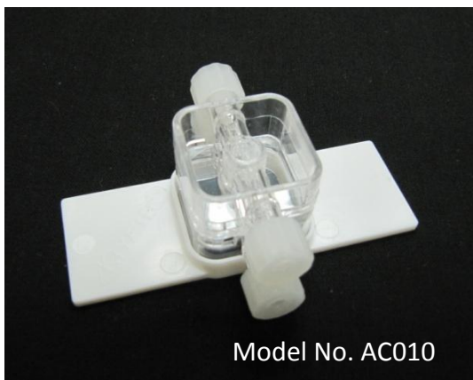
(Left) Universal Stage Adapter with capped 3DKUBE. (Right) In situ 3D confocal image of MCF7 breast cancer cells in alginate beads (100x total magnification).
